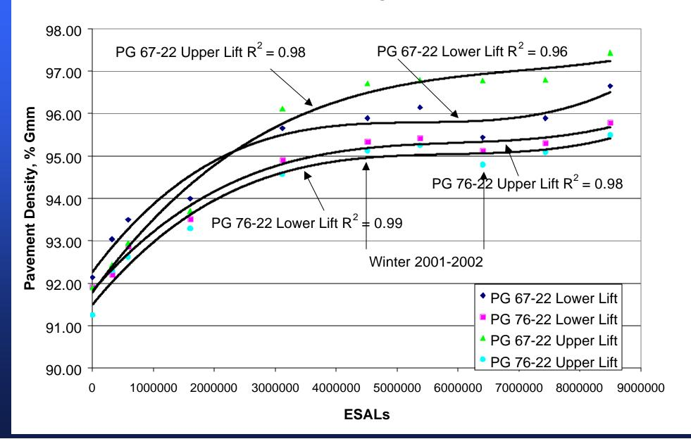
Estimation of Density at a Given Gyration Level Density at Gyration X ? Density at NDesign ? <u>Height at NDesign</u> Height at Gyration X NCAT Test Track - Design Gyrations to Meet Pavement Density
